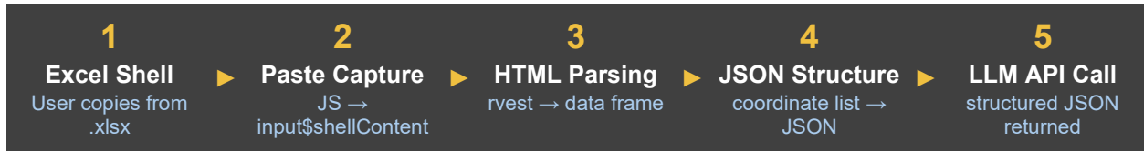
Figure 2. Shell Annotation Pipeline: Three Deterministic Stages (Programs 2–4) Followed by LLM Inference (Program 5)
