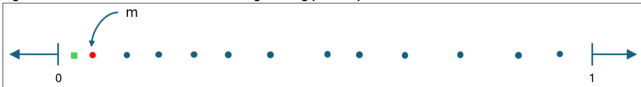
Figure 12. Number line of exact values using floating point representation
